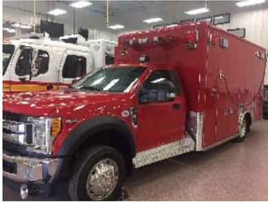
The new chassis is a 2017 Ford F550 and features a liquid spring suspension system. It provides a very smooth ride and aids in the handling of a typically top-heavy vehicle. In addition to the new chassis, the entire unit was gone through and refreshed where possible.
